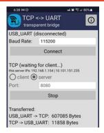
Essentially, TCPUART connects to the Nano/Tiny SA via USB. It then magically encapsulates the data so it can be sent via TCP/IP out the Wi-Fi server in TCPUART.
