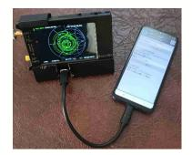
To continue setting up TCPUART, make sure the baud rate is 115200 and press 'Connect'. The label will change to 'Disconnect' which actually means you are connected. Your Cell Phone will likely ask you if you want to give TCPUART the right to rummage around in your phone so it can find a device. Answer 'OK'.
